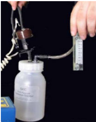
Figure 5-2a. Haz-Dust IV sensor connected to CH-103 calibration chamber.
