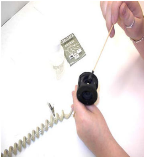
Figure 5-6. Sensor head being cleaned with cotton swab.
