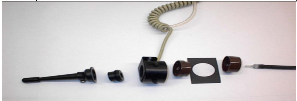
Figure 3.3. Component identifications from left to right: SKC GS-Cyclone for Respirable sampling, GSA-202 adapter, sensor head, disassembled filter cassette, filter, and air intake tubing.
