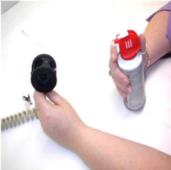
Figure 5-4. Dust being removed with low pressure air.
