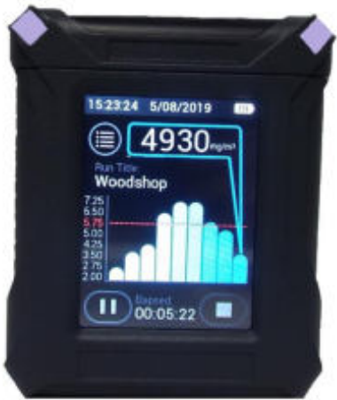
Figure 3-16. Flow Faults cause purple lights to flash
