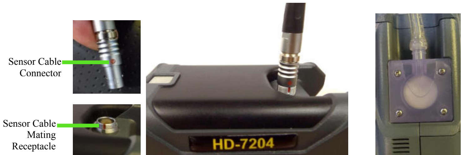
Figure 3-1. Sensor Cable being connected to HD-7204 and tubing connected to air intake
