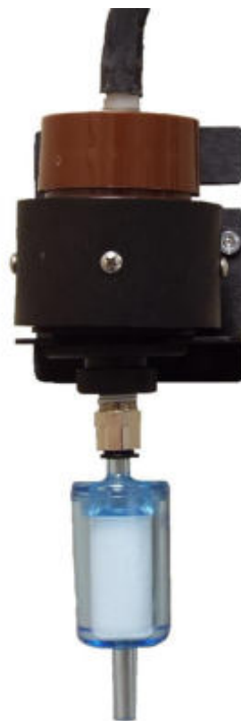
Figure 3-14. Zeroing filter (p/n ZA-7204) attached to the IOM Inlet.
