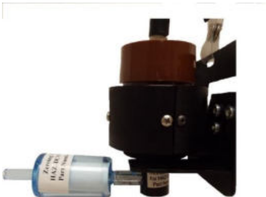
Figure 3-13. Zeroing filter (p/n ZF-102) being attached to the Thoracic sampling inlet.
