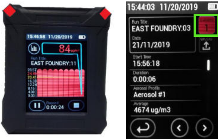
Figure 3-17. Battery Faults cause red lights to flash
