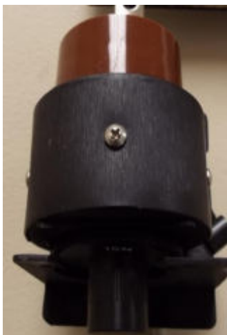
Figure 5-1. CS-7204 being inserted into HD-7204 sensor
