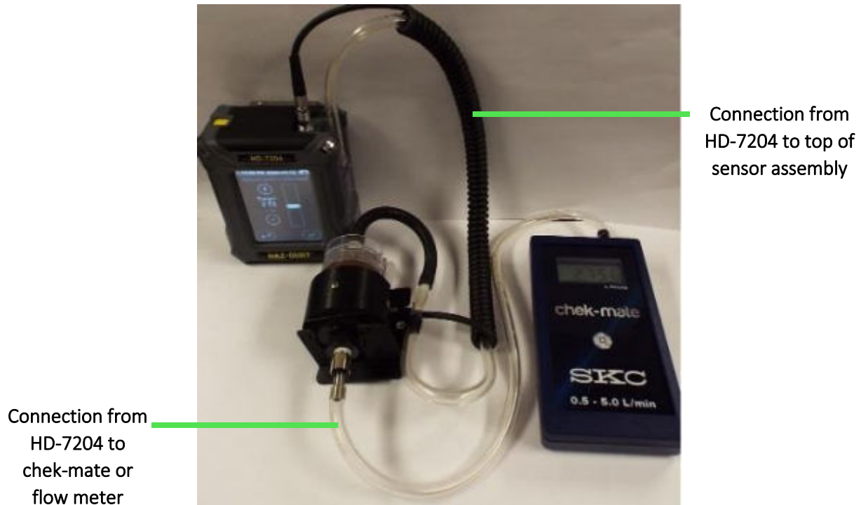
Figure 3-12. Connecting HD-7204 to SKC chek-mate
