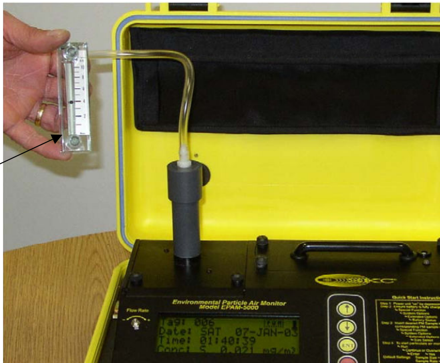
Figure 5-2. Flow Adjustment Meter attached to EPAM-5000.
