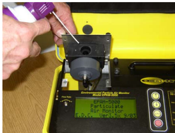
Figure 5-6. Dust being removed with low pressure air.
