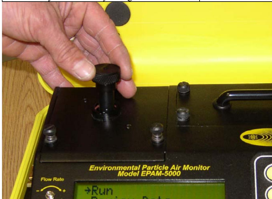
Figure 5-1. Inserting CS-105 into SKC EPAM-5000 Sensor.
