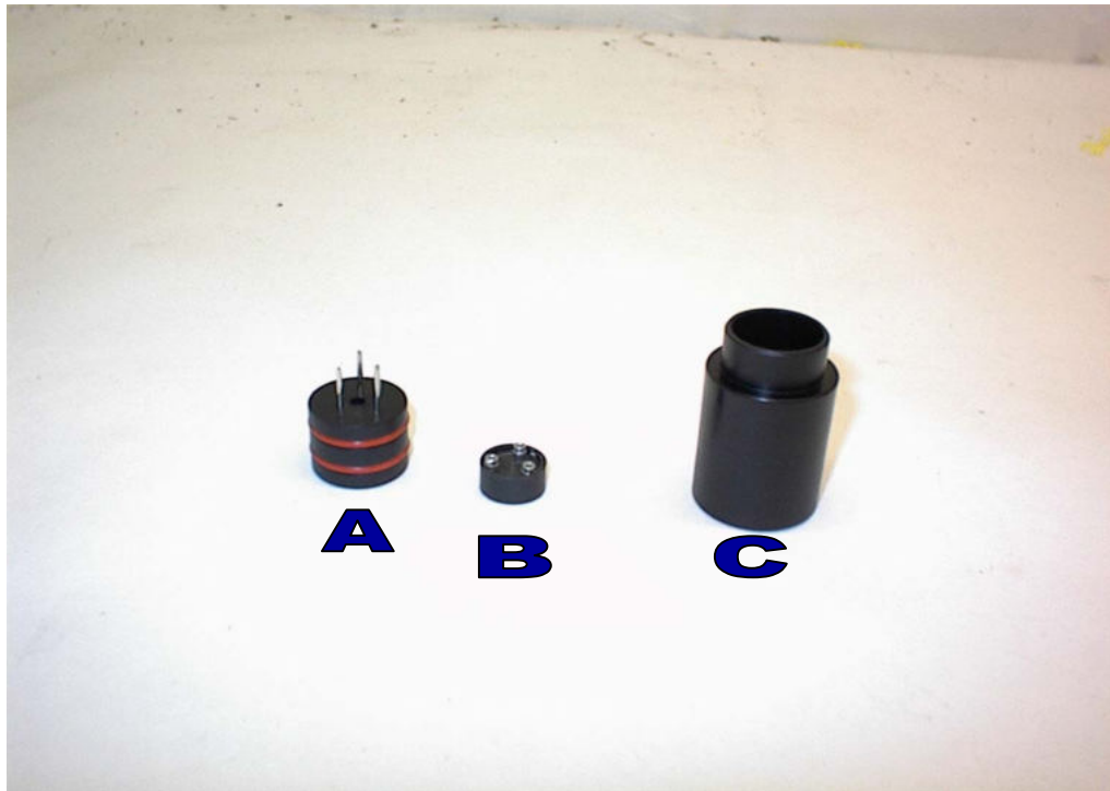
Figure 3-1. Picture: A) Impactor Jet, B) Impaction cup, and C) Impactor Sleeve. For TSP sampling use impactor sleeve without impactor. One Size Selective Inlet is provided with EPAM-5000. Impactors are engraved on bottom of jet.
